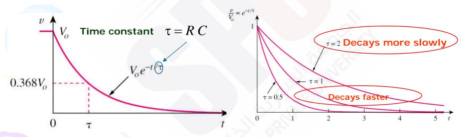
• The time constant  $\tau$  of a circuit is the time required for the response to decay by a factor of 1/e or 36.8% of its initial value.
